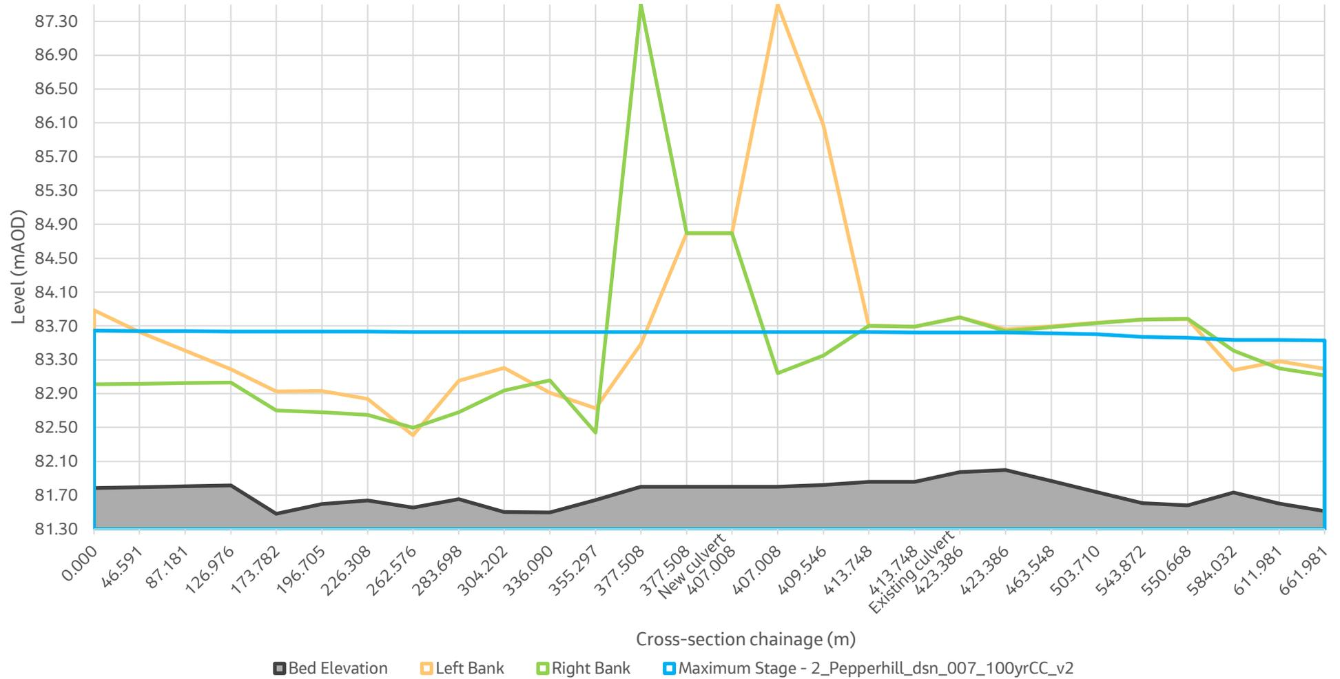
Figure 10: Maximum Water Level profile predicted for a 1 % AEP Event plus Climate Change for the scheme scenario on the Pepperhill Tributary
