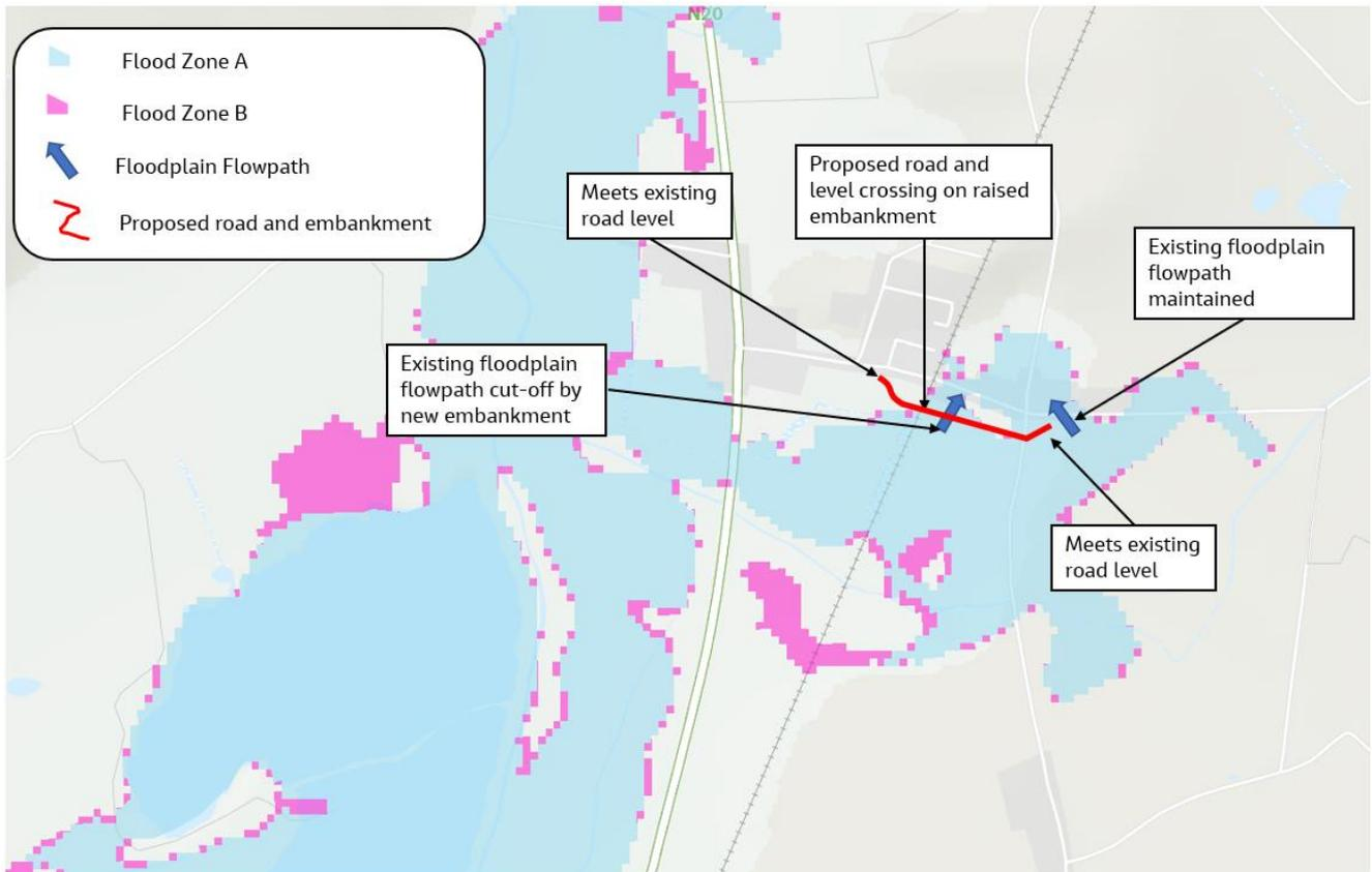
1% AEP flood levels in the area can be estimated to be maximum 95.7mOD based on the available flood extents. This compares to the finished ground levels for the Proposed Project vary but are typically greater than 98.0mOD throughout. This indicates that the Proposed Project will not be at risk of flooding.
