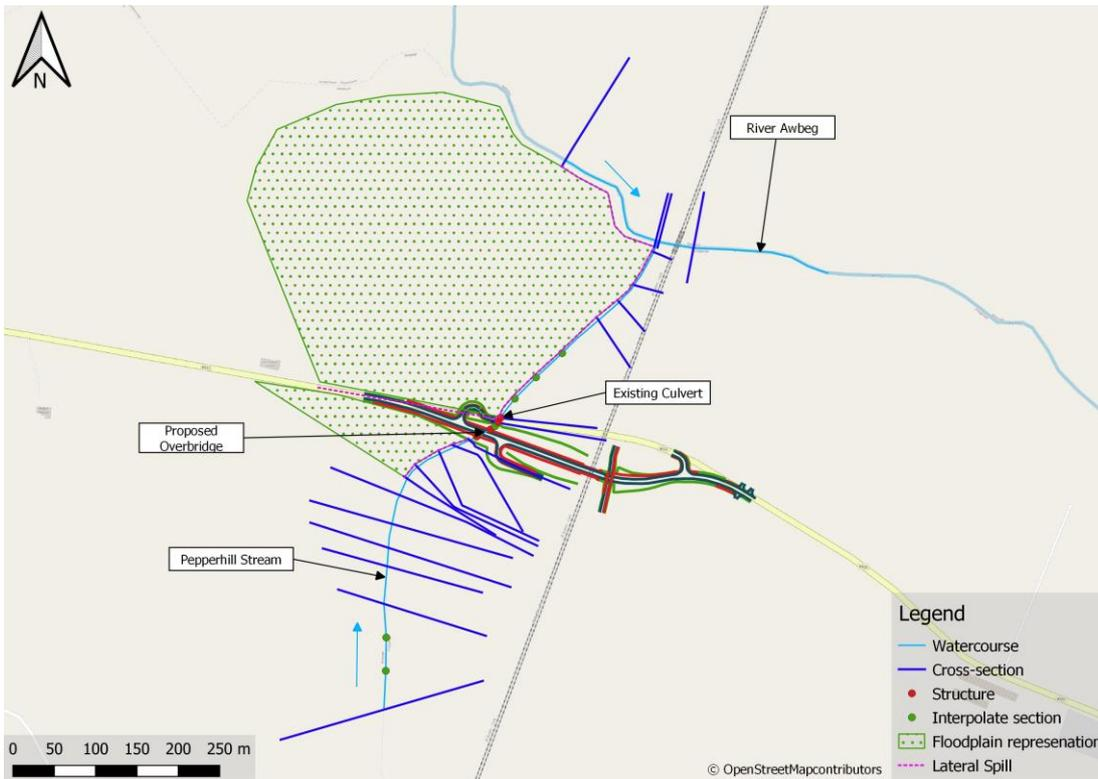
Figure 4: Scheme Scenario (new bridge with box culvert)
