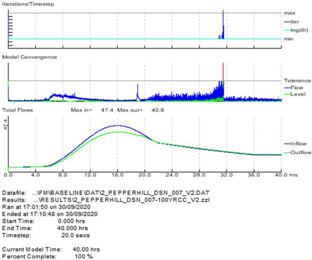
As the Pepperhill Stream is ungauged and no gauging stations are located on the River Awbeg in the vicinity of the modelled reach, no hydrometric data was available for calibration/validation purposes. Cork County Council provided a map of observed flood extents for the Buttevant area. This mapping was used to verify the results of the baseline 1% AEP flood event and a plan showing good verification between the two can be seen in Inset Figure 1.13 below.
