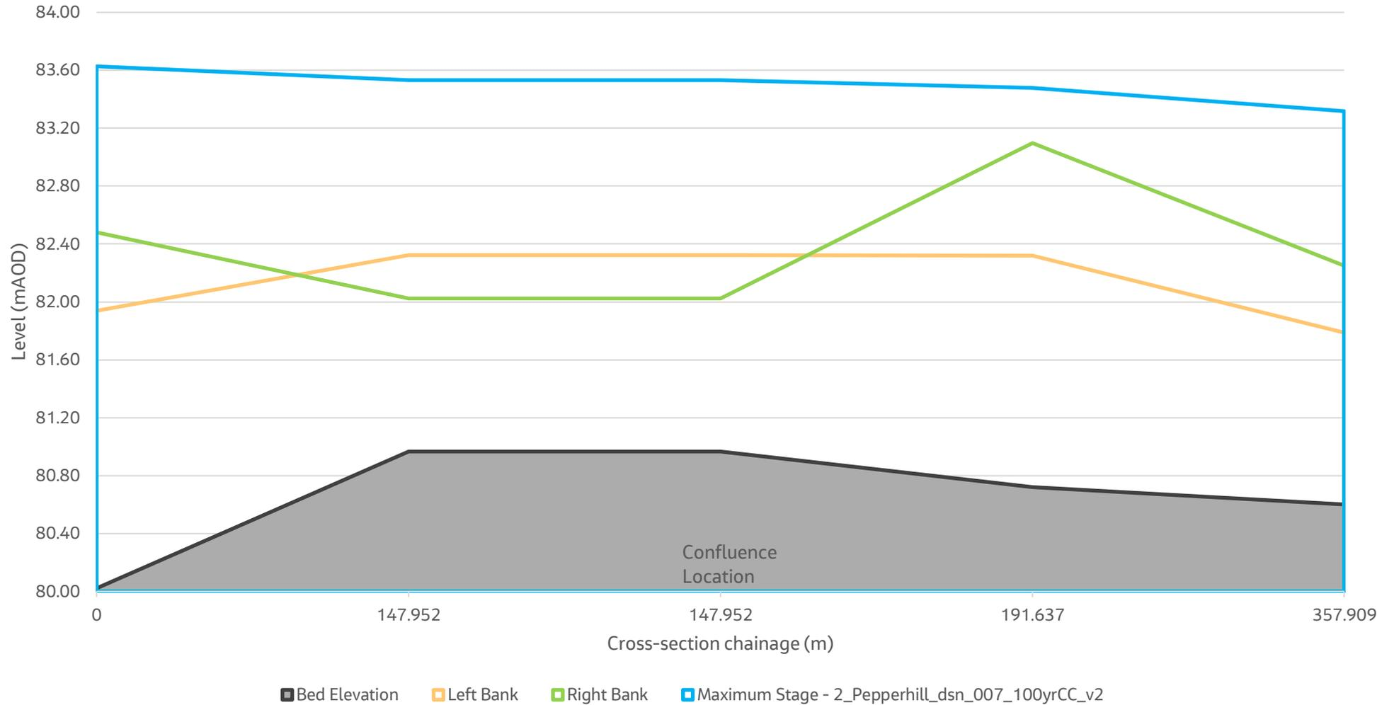
Figure 11: Maximum Water Level profile predicted for a 1 % AEP Event plus Climate Change for the scheme scenario on the River Awbeg
