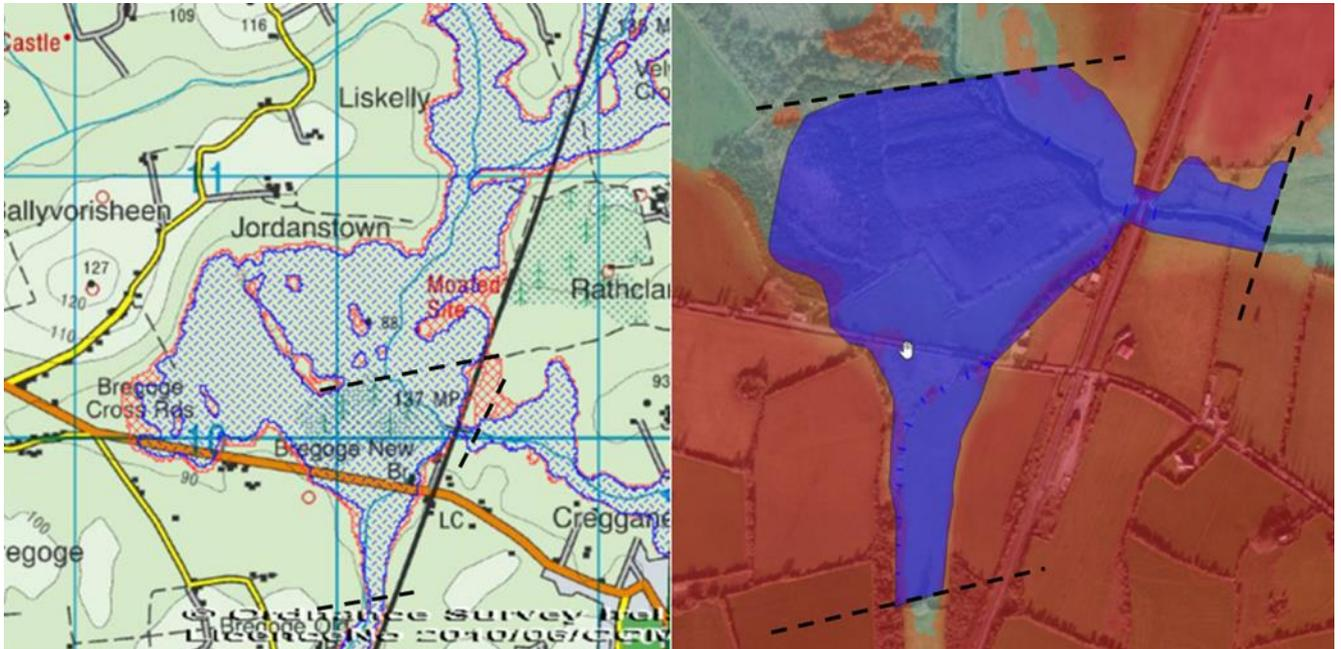
Model boundaries in Inset Figure 1.13 are illustrated in dashed black lines, flood extents illustrated in blue, red shading on right hand side shows higher ground based on LiDAR
