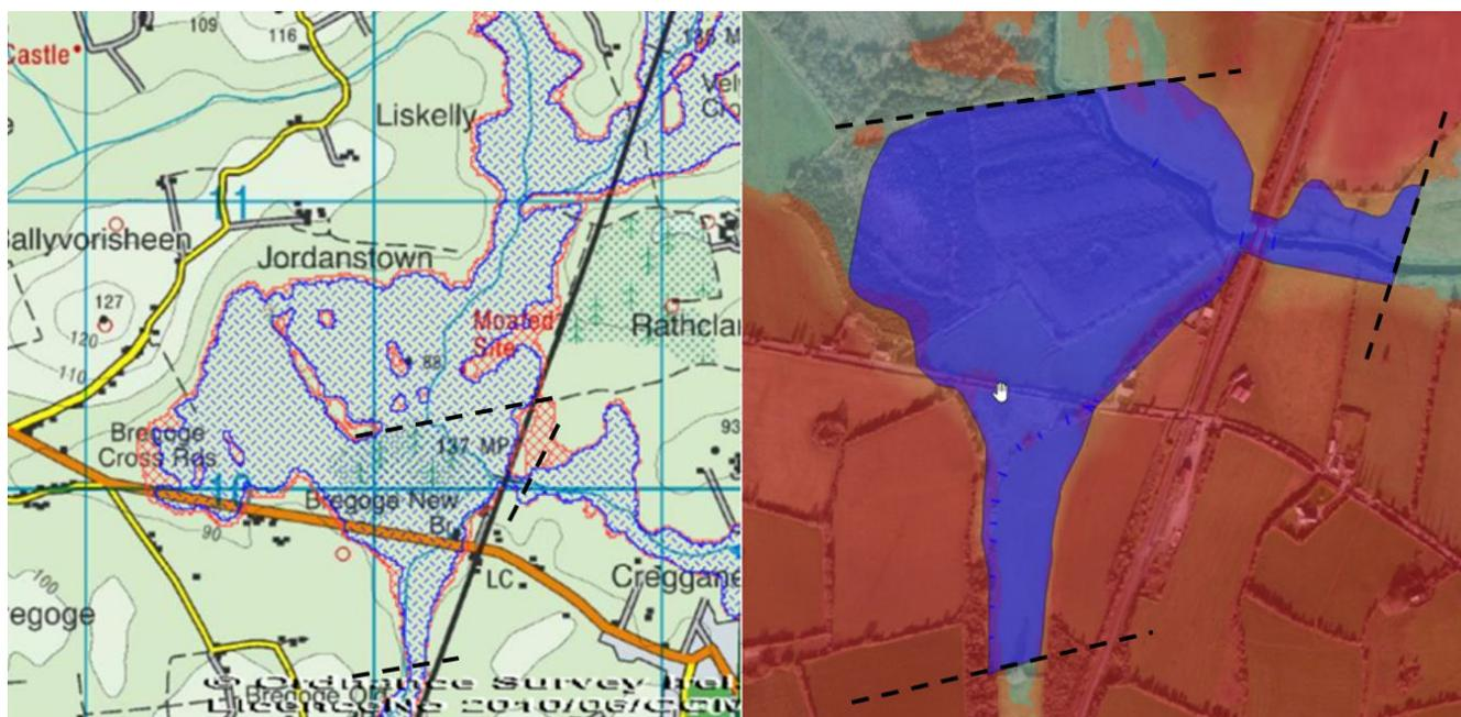
Figure 7: Comparison of observed flood extents from Cork County Council (left) and modelled flood extents (right)
